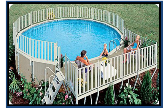
Appropriate fencing with pull-up stairs
